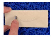
Take the back side of the instrument, the convex surface and place onto the stone. Raise the angle of the instrument up to approximately 45 degrees, so the back of the tip of the blade touches the surface of the stone.
