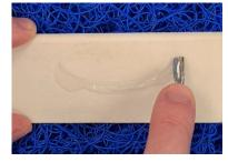
Draw the instrument from right to left in the shape of the "U" back and forth, pressing hard enough to see metal filings on the stone.
