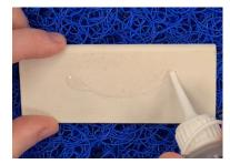
Drip a small amount of oil (**MD30**) onto the flat surface of your stone in the shape of a smile or a shallow "U" shape.
