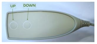
The height of iM3 Shona is adjusted by a wired hand control. The upper button raises the table and lower button lowers the table.
