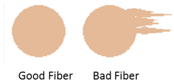
Figure 3.11 Aiming beam spot emitted from good fiber compares with that from bad fiber
