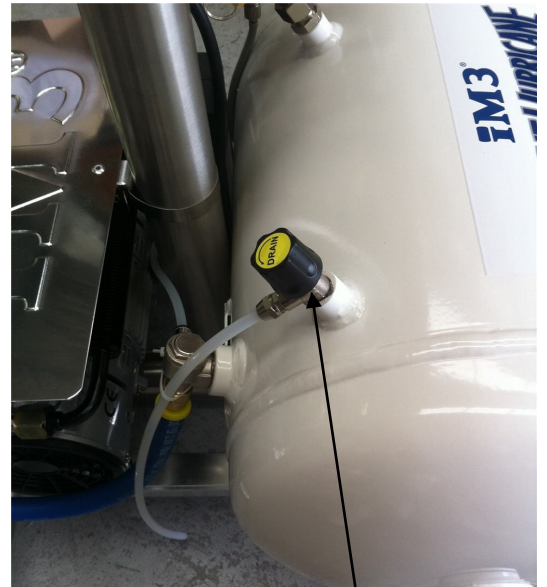
Compressor tank drain, located on top of white air tank— open slowly Place container under white tube to collect
