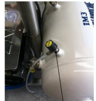
Compressor tank drain, located on-top of white air tank—open slowly Place container under white tube to collect water.
