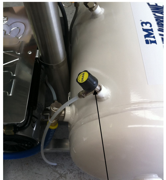
Compressor tank drain, located on-top of white air tank— open slowly Place container under white tube to collect water.
